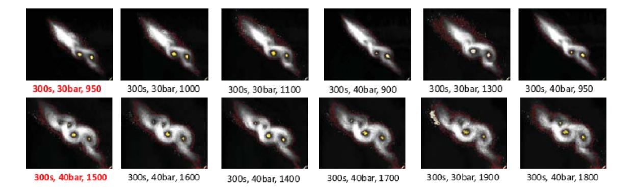
Spray vortex analysis in combustion engineering: compare experiments with simulations
